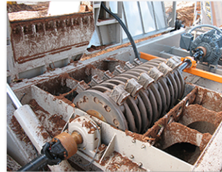
46" Hammermill & Two Electric Motors shown on a TCII-1564SE
