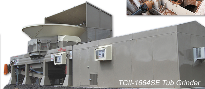
46" Hammermill & Two Electric Motors shown on a TCII-1564SE
