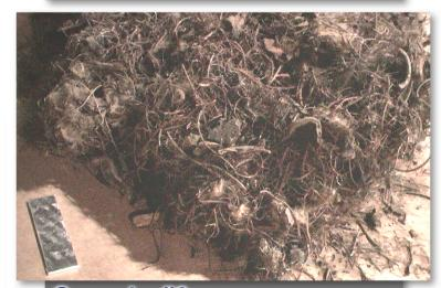
**Sample #3** - Through 1 ½" screen. Can be reground to remove more metal. Result is Fluff (Metal, Nylon & Rubber Mix).
