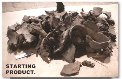
Sample #1 - Approx. 4" chips from Slow Speed Primary Shredder.
