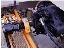
When the load on the hammermill increases, the hydraulic fluid is automatically re-routed against the turbine blades, adding approx. 30% additional reaction torque to engine torque. The engine is protected by the torque converter fluid absorbing shock loads & torsional vibrations from the hammermill, assuring longer engine life.
