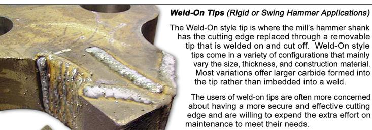
Being required to cut off old tips and weld on new tips requires more time and labor than some other alternatives. The maintenance technician is required to be a skilled metal worker and welder with welding equipment, but when done properly the tip retention is very solid on this 2-piece arrangement.
