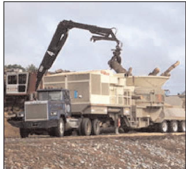
An operator uses a Hood loader to place logs into this grinder to begin P.R. Russell's mulch manufacturing process.
