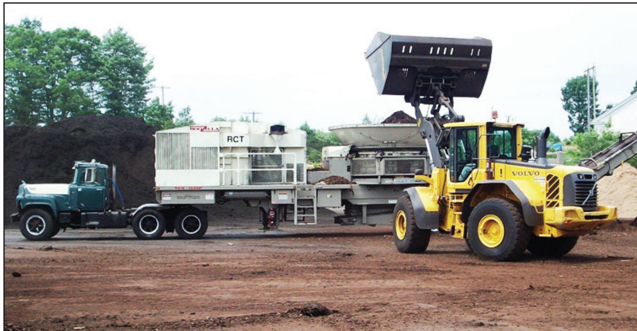
An operator backs his Volvo loader away from one of P.R. Russell's TCII-1564 Hogzilla grinders that is regrinding mulch.
