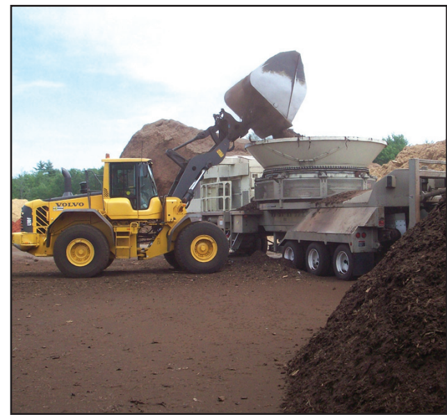
An operator dumps a load of material into this grinder.
